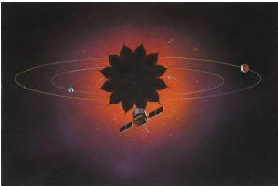
Artist's concept of the New Worlds Observatory. The dark, flower-shaped object in the center is the star shade. (Credit: NASA and Northrop Grumman)
