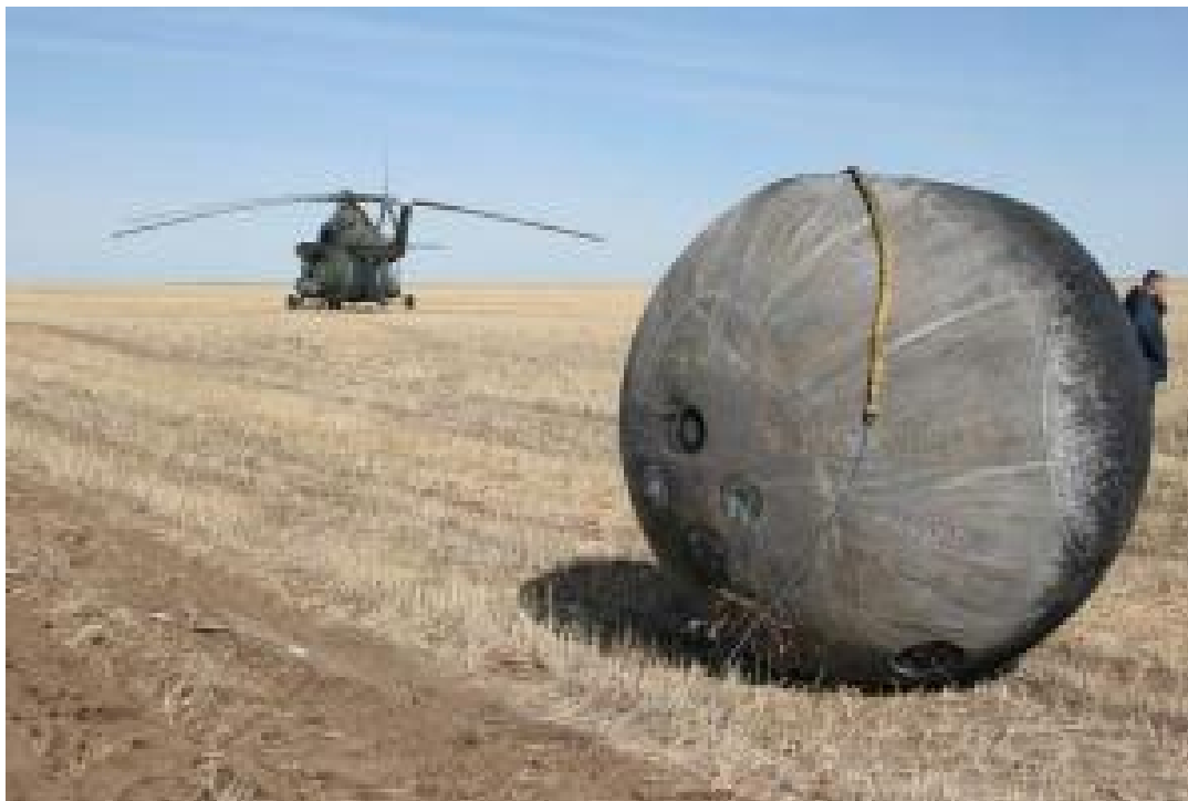
The Foton-M3 capsule immediately after landing. The STONE-6 rock samples were fixed in the circular positions at the left side of the capsule. (Credit: Image courtesy of Europlanet)
